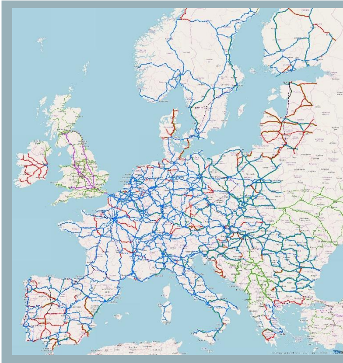
Figure 8: TEN-T network corridors compliance map for electrification of railways. Tracks compliant with guidelines on electrification (i.e., electrified lines) are shown in blue, non-compliant lines in red, lines with no compliance data are black. Further lines of the core (green) and comprehensive (purple) network for which no KPI compliance assessment is performed, are included (Retrieved from the TENtec Interactive Map Viewer on 03/24/2022).
