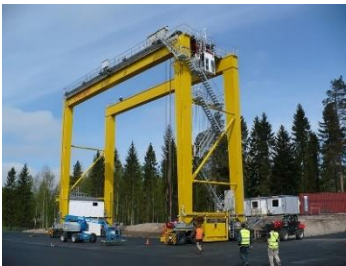
Figure 7: Rubber tyred gantry crane (“RTG aka Rubber tyred gantry crane by Konecranes in Finnish factory at Hyvinkää test site” by Derek Yu, CC BY 2.0)
