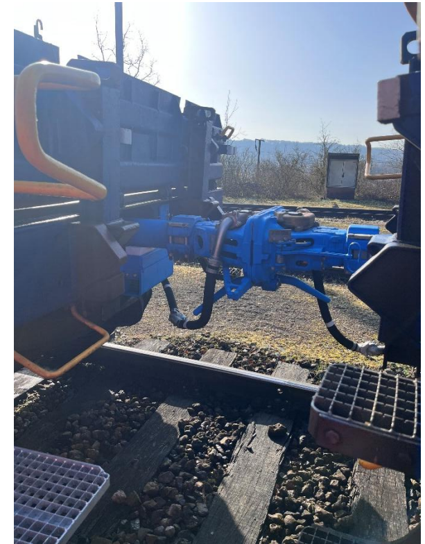
DAC operational validation test in Belval March 2026
